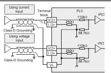
\*1 Make sure to short-circuit the 'V□+' and 'I□+' terminals when current is input. (□: input channel number)
